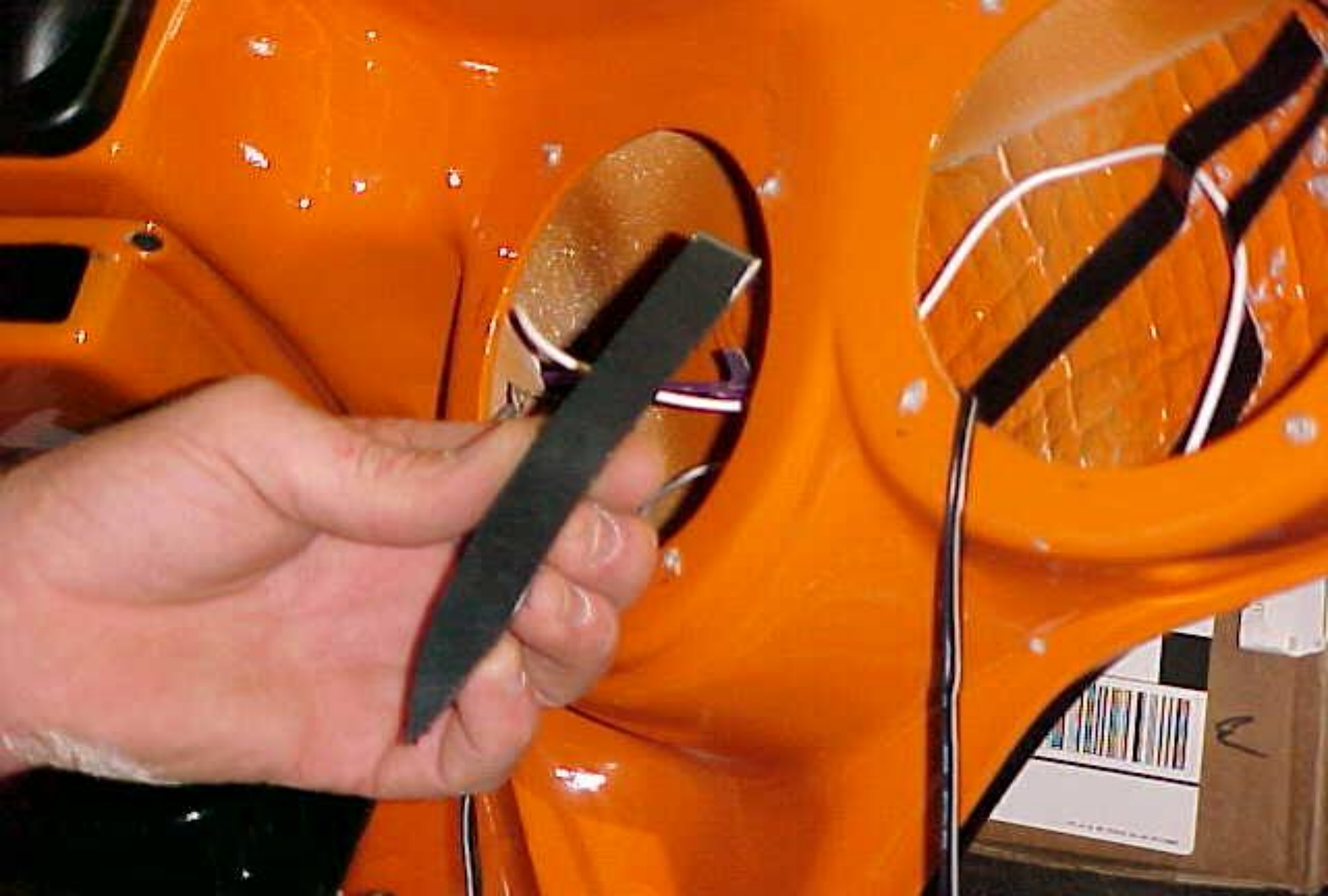
Take the reinforcement piece and place inside fairing along the inside edge.
